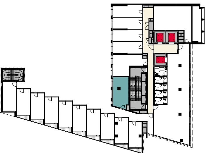
LEVEL 02 STUDIO SOUTH Floor area: 24m 2 Floor area exc kitchen & bath: 19m 2 (Compliant: SEPP Part 3, 69(1)(a) )
