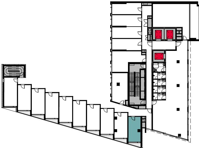
STUDIO (SOUTH) ROOM Floor area: 17m 2 Floor area exc kitchen & bath: 12m 2 (Compliant: SEPP Part 3, 69(1)(a) )
