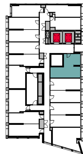
LEVEL 03 ACCESSIBLE ROOM Floor area: 26m 2 Floor area exc kitchen & bath: 17m 2 (Compliant: SEPP Part 3, 69(1)(a) )
