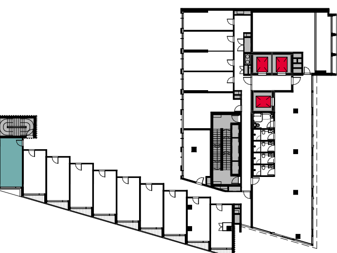
LEVEL 02 STUDIO ROOM Floor area: 20m 2 Floor area exc kitchen & bath: 15.5m 2 (Compliant: SEPP Part 3, 69(1)(a) )
